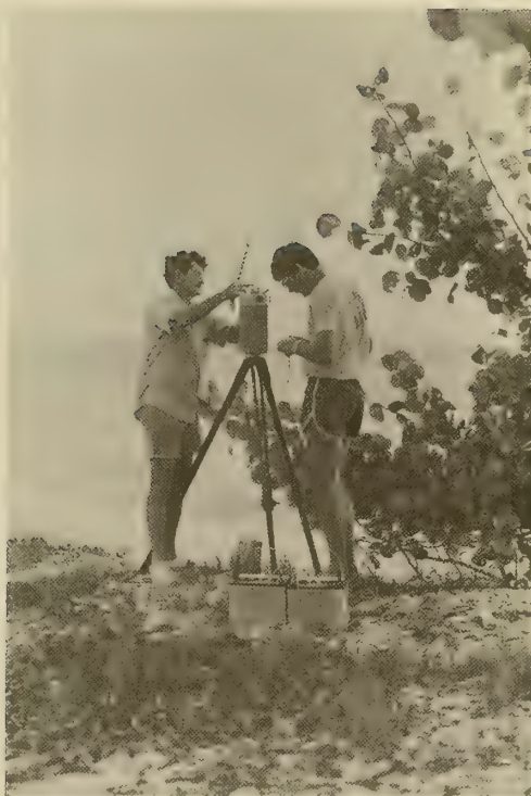
Figure 3. Trisponder shore location being installed in preparation for an offshore survey.
